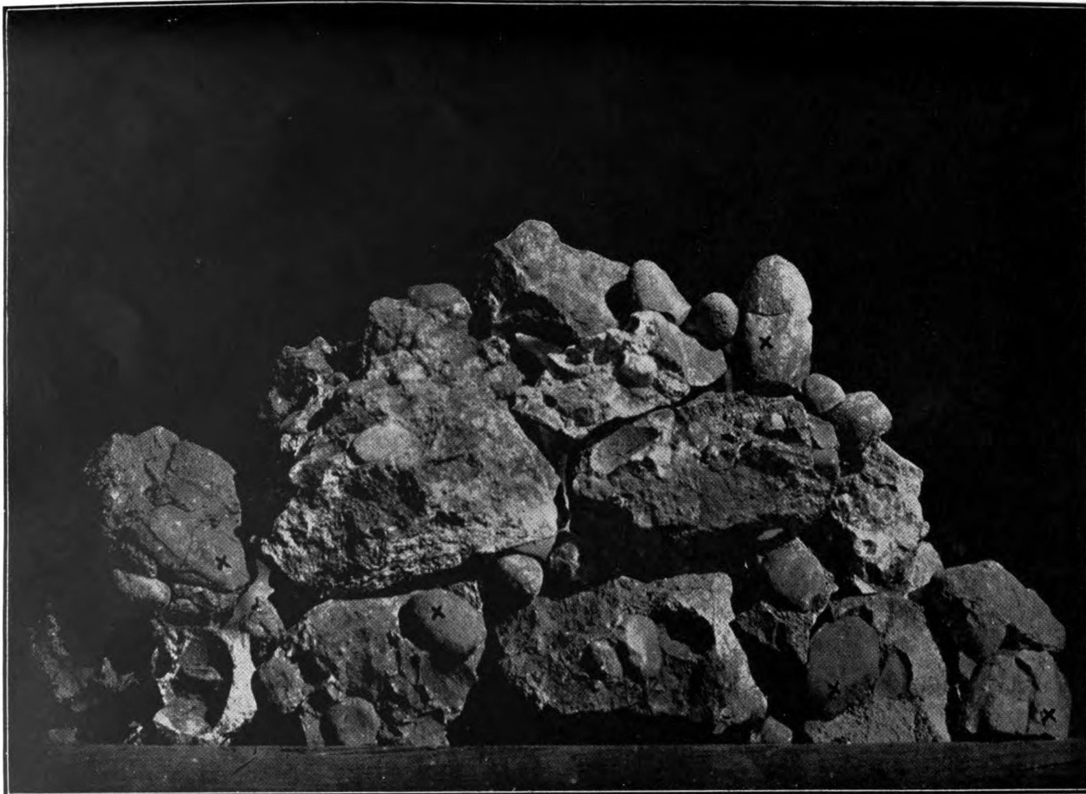
(5) Van Ryn Reef, upper portion, outcrop specimen from Van Ryn Estates—New Modder outcrop. This Reef body is known on these mines as the "Egg Shaped Pebble Reef." Egg shaped pebbles marked x. (Photograph scale \frac{1}{2} linear actual size.)
