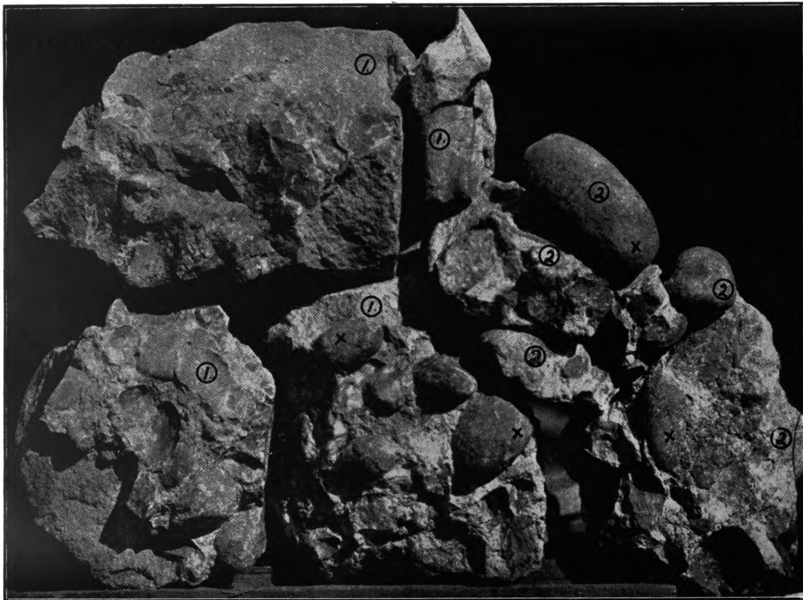
(6) Van Ryn Reef, upper portion (the "Egg Shaped Pebble Reef"): (1) from Klippoortje (Houtpoort, Ltd.); (2) from Heidelberg Townlands (Eastern Van Ryn and Modderfontein G.R., Ltd.). Egg shaped pebbles marked x. (Photograph scale \frac{1}{2} linear actual size.)
